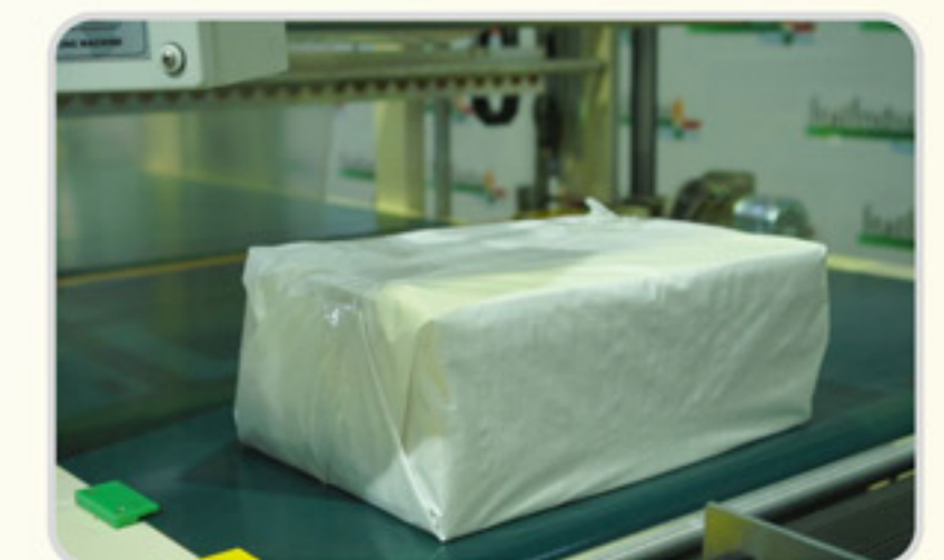
Stacked reams wrapped with HDPE sheet
